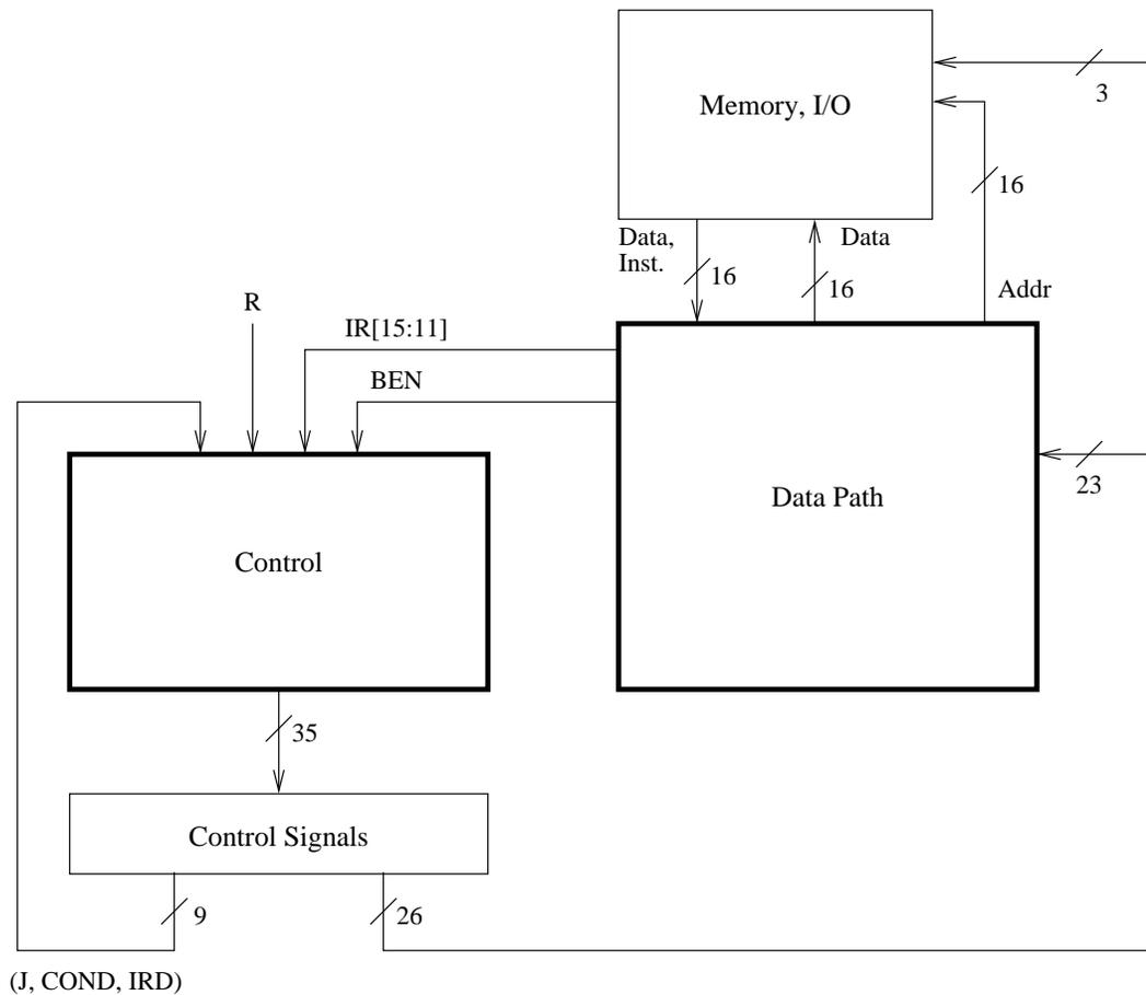
Figure C.1: Microarchitecture of the LC-3b, major components
