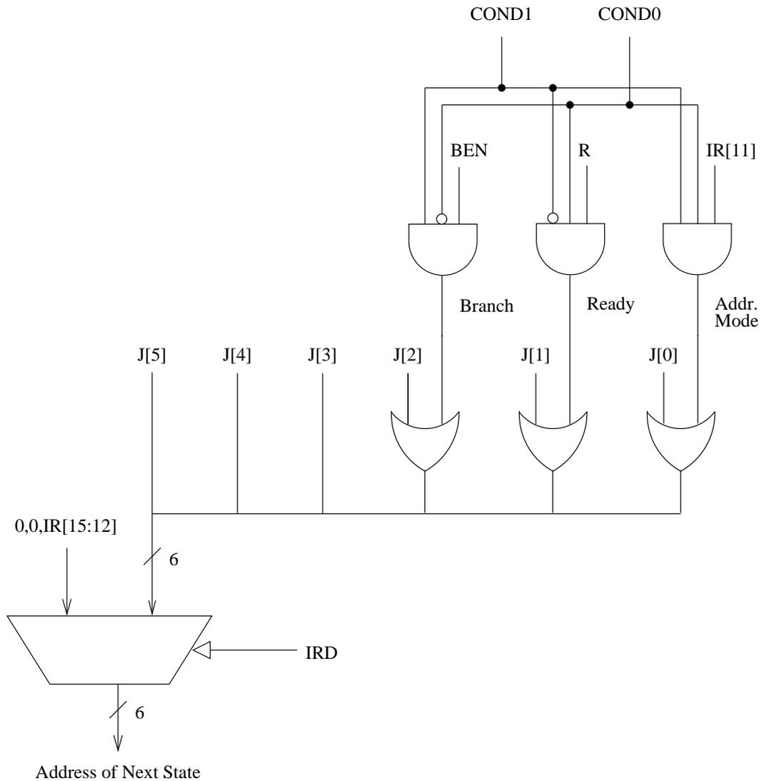
Figure C.5: The microsequencer of the LC-3b base machine
