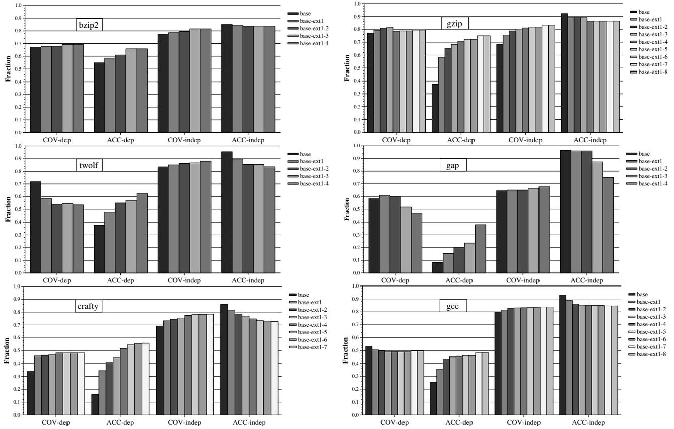
Figure 17. Per-benchmark accuracy and coverage of 2D-profiling when a perceptron predictor is used in the target machine
