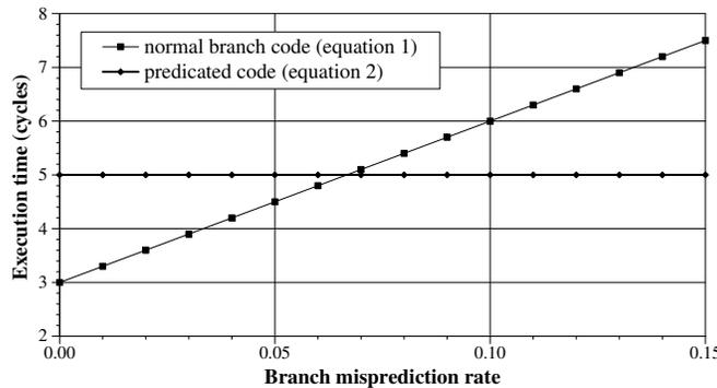
Figure 2. Execution time of predicated code and non-predicated code vs. branch misprediction rate
