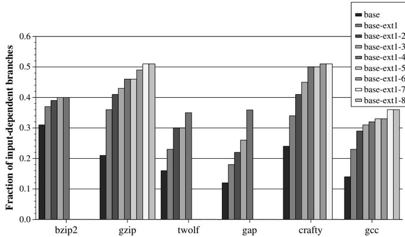
Figure 13. Fraction of input-dependent branches when more than two input sets are considered
