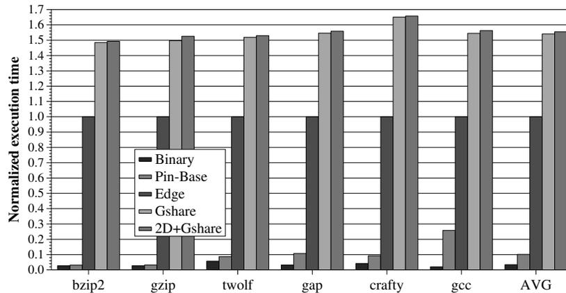
Figure 22. Overhead of 2D-profiling compared to edge profiling
