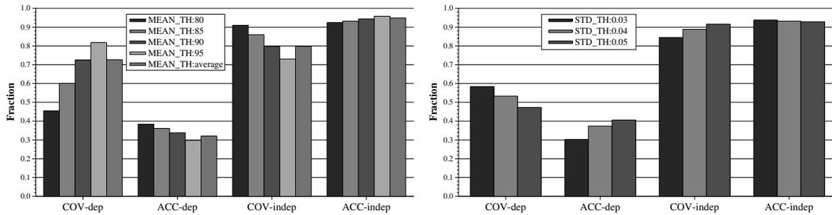
**Figure 12. Threshold sensitivity of coverage and accuracy**
