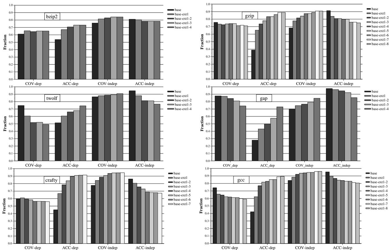
Figure 14. Per-benchmark accuracy and coverage of 2D-profiling when more than two input sets are considered
