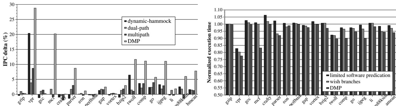
Figure 12. Performance comparison of DMP versus other paradigms on the less aggressive processor
