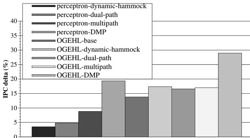
Figure 13. DMP performance with different branch predictors
