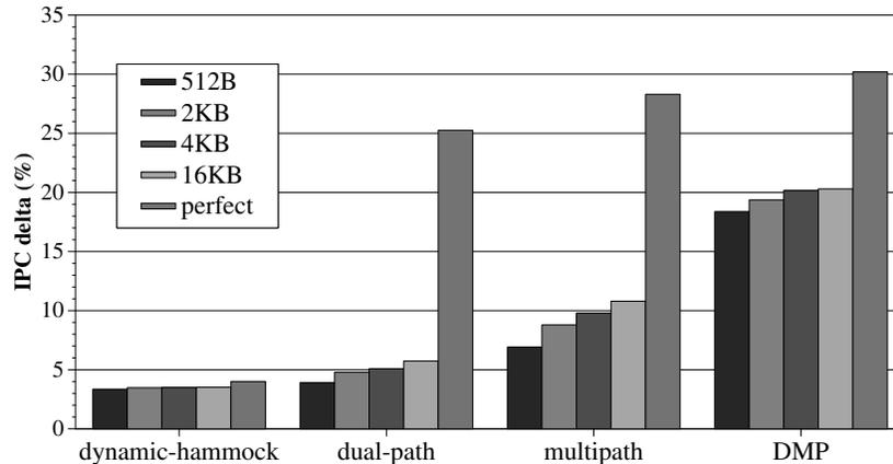
Figure 14. Effect of confidence estimator size on performance
