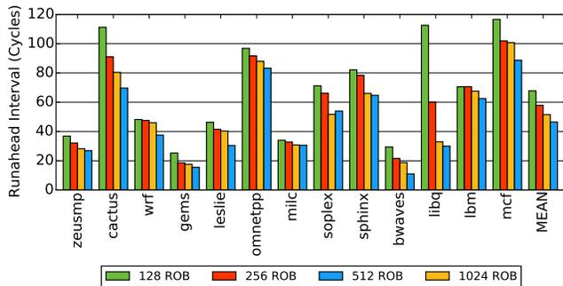
Figure 3: Average number of cycles per runahead interval.
