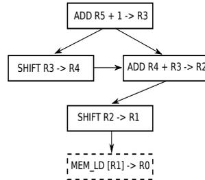
Figure 4: Example dependence chain adapted from *mcf*.
